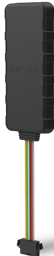
HYN001 is a well designed LTE Cat.1 GPS tracker used for all kinds of vehicle tracking applications. It has built in BLE and backup battery. The multiple I/O interface support various external sensors. Also the compact size ensures conceal and easy installation. The HYN001 has good quality and excellent GPS performance, it has passed major operators certifications in the world.
